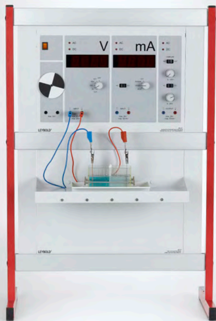
The electrochemical series (C4.4.3.1_a)
