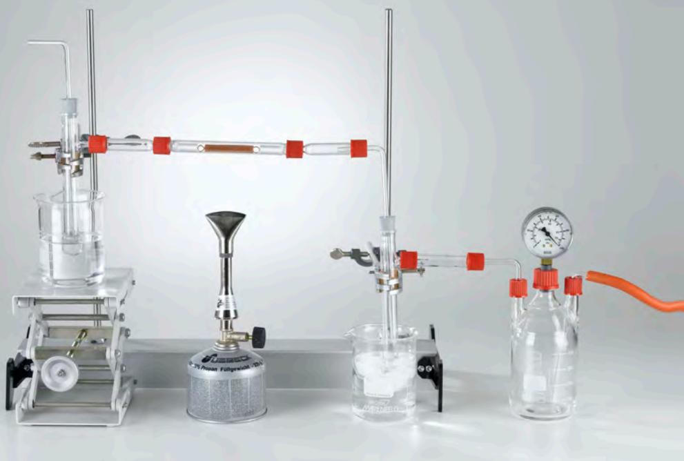
Oxidation of propanol (C2.2.2.1)
