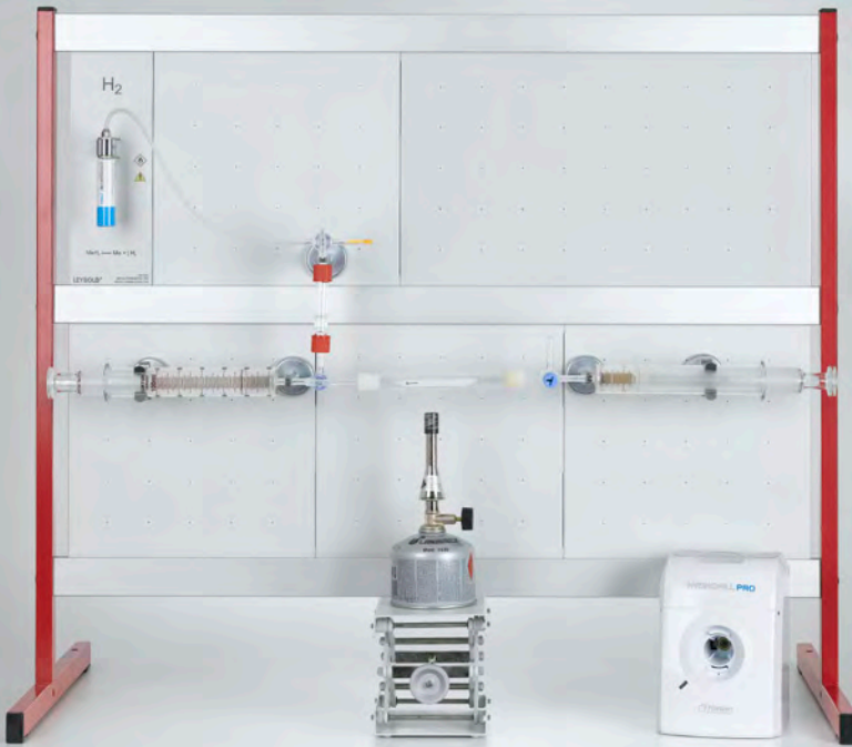
Synthesis of ammonia by the Haber-Bosch process (C5.1.1.2)
