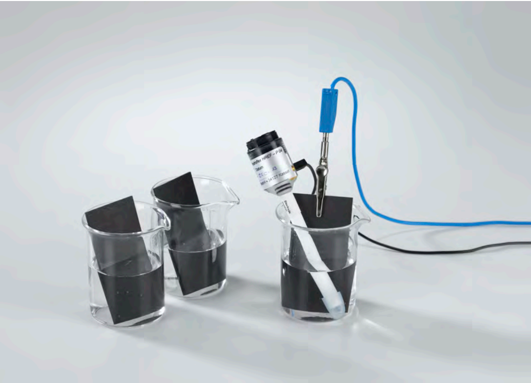
Standard potentials of non-metals (C4.4.3.3_b)
