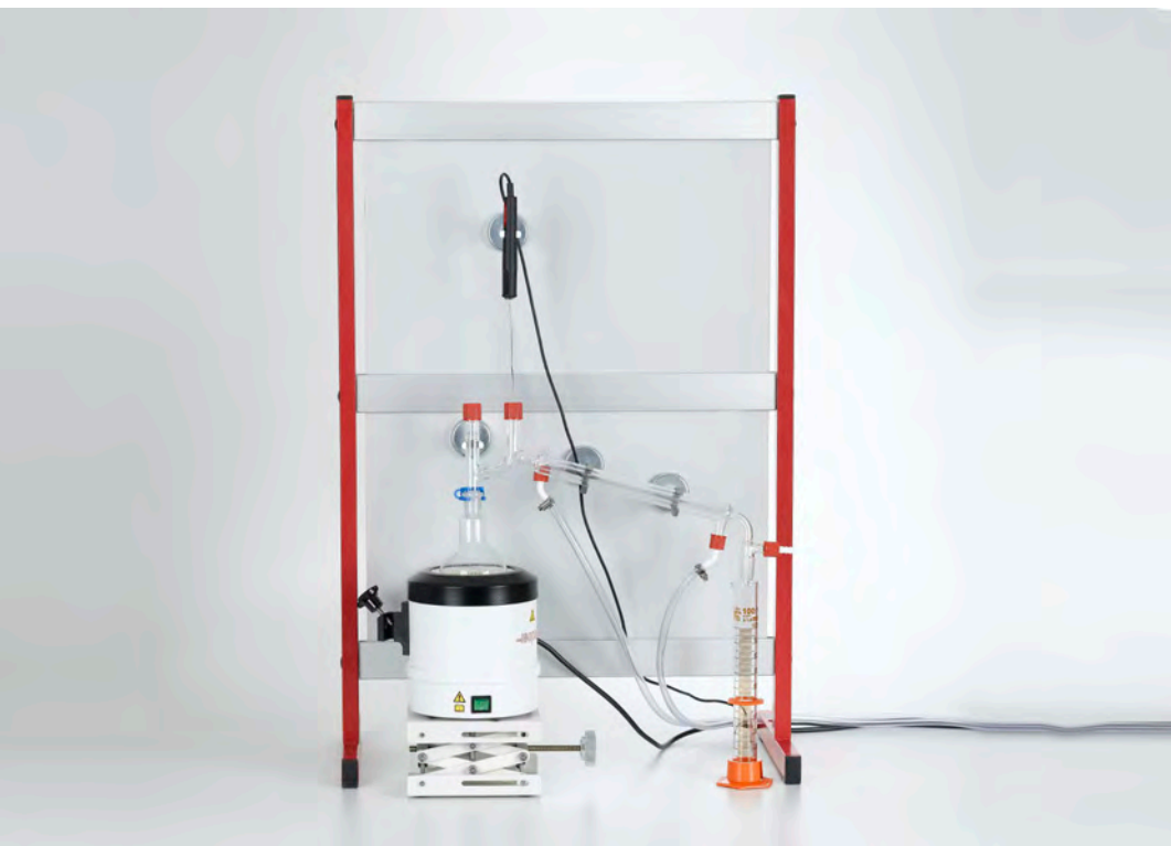
Boiling range distribution of petrol (C2.3.3.1)
