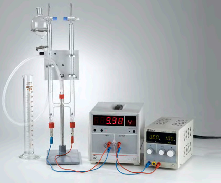
Determination of the Faraday constant (C4.4.5.2)
