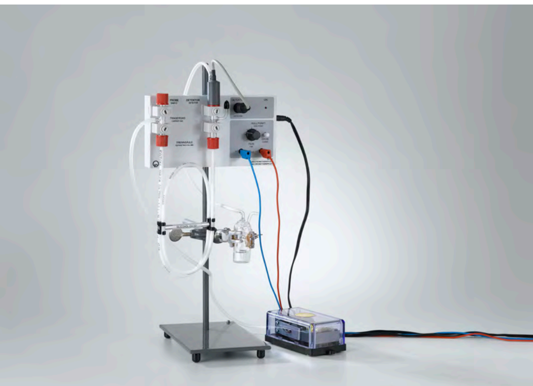
Gas chromatographical analysis of cigarette lighter gas (butane gas) (C3.2.1.1)
