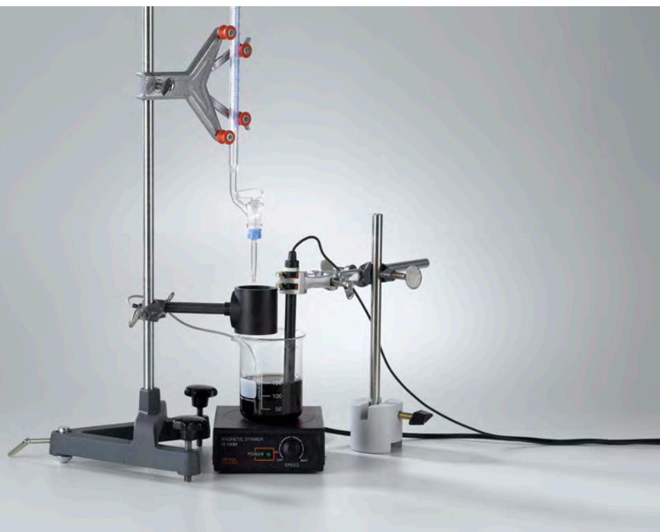
Determination of the content of phosphoric acid in a cola drink (C3.6.4.2)
