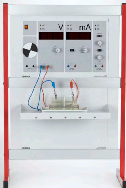
Concentration potentials (Nernst equation) (C4.4.3.4)
