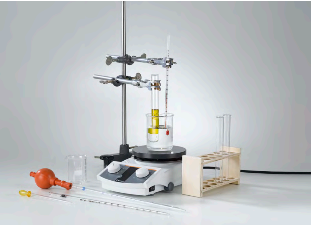
Production of fuel from rapeseed oil (C5.4.1.1)
