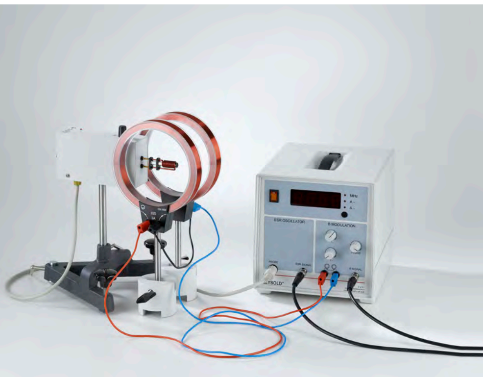
Electron spin resonance on DPPH (C3.4.4.1)
