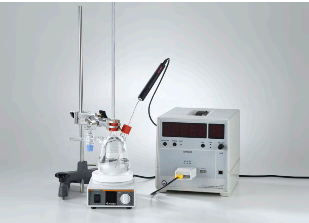
Thermal anomaly of water (C1.3.3.1)
